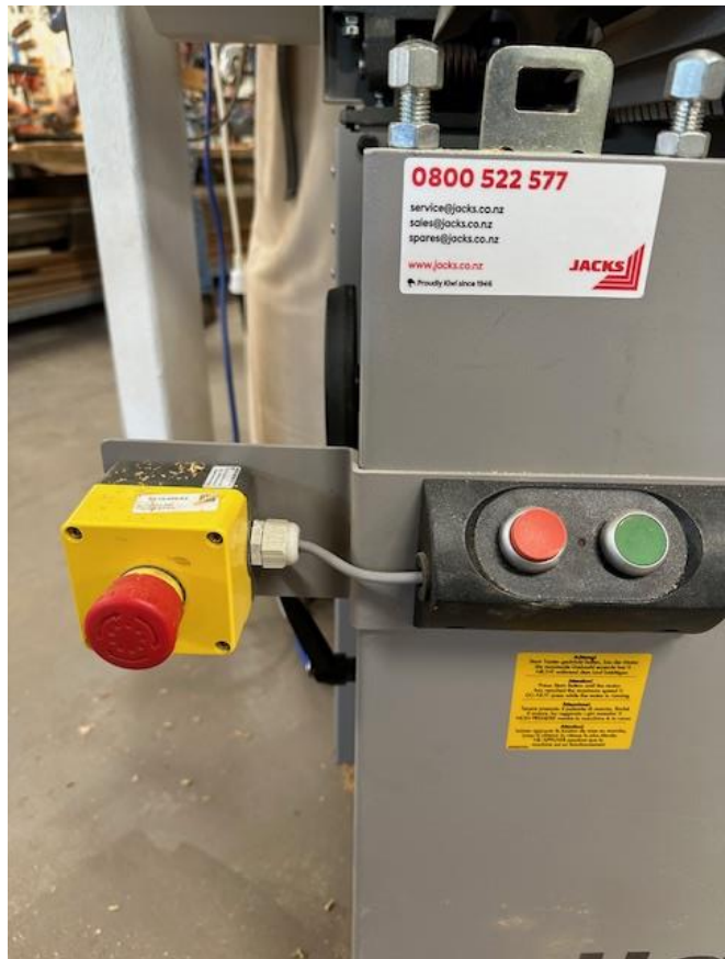
Now we have an emergency stop button
