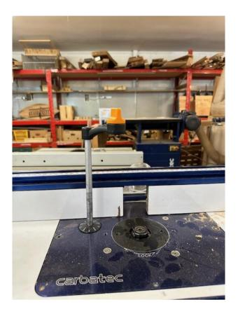
To stop the router breaking again we have removed the locking lever. The round adjusting handle is not to be used to move cutting head up and down this is designed to be used when plunge cutting (which you obviously can't do when router upside down and fixed to table).
